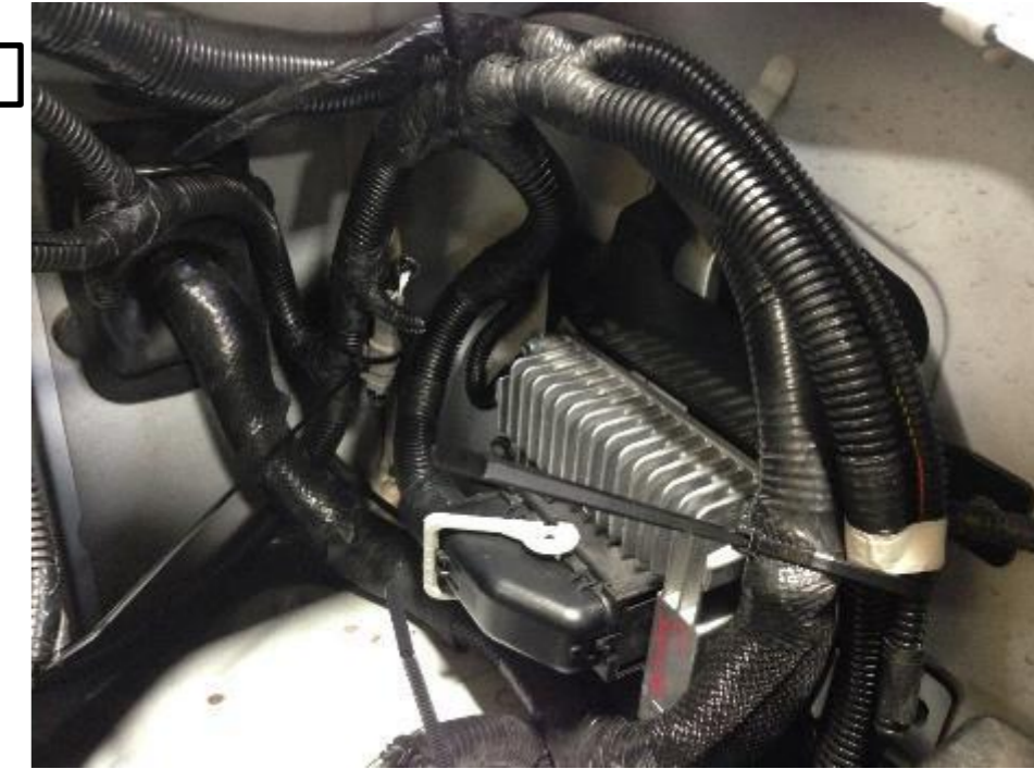
A – M6 x 1.0 x 16 bolt Tighten to 8–12 Nm. B – M6 x 16 self tapping screw
